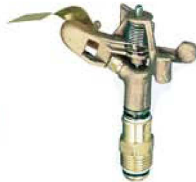
7250 - Brass Full Circle \frac{1}{2} " Male pipe thread connection. Anti-splash arm reduces backsplash. Pack: 10/80 (Carded)
